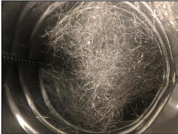
**Fig. 2.** A view of aluminum wool used in the solar heating systems
