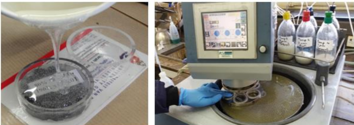
Figure 3 Preparation of sinter samples for mineralogical researches.
