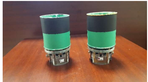
Figure 1. Two E-puck robots that are used in the experiments. As can be seen in the figure, the robots are fitted with a colorful hat to make it easier for them to detect each other.
