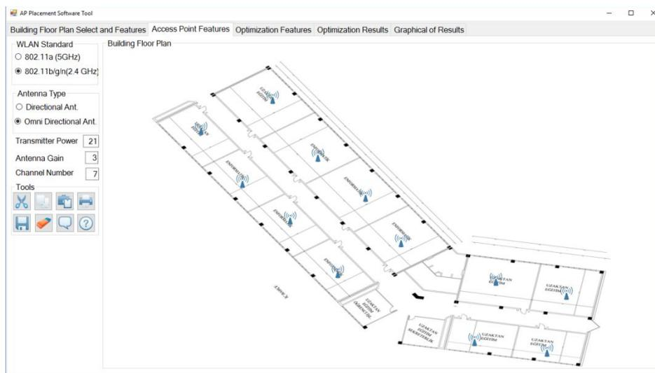
**Figure 6. Access Point Features Module**
