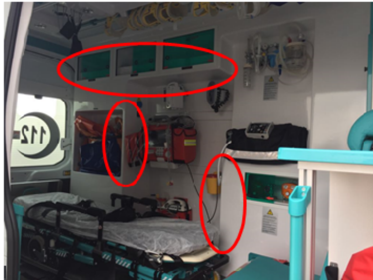
Figure 2: Sharp corners in the cabin.
