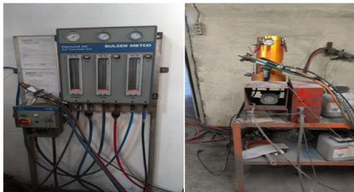
Figure 2. Plasma spray coating system that used for coating
