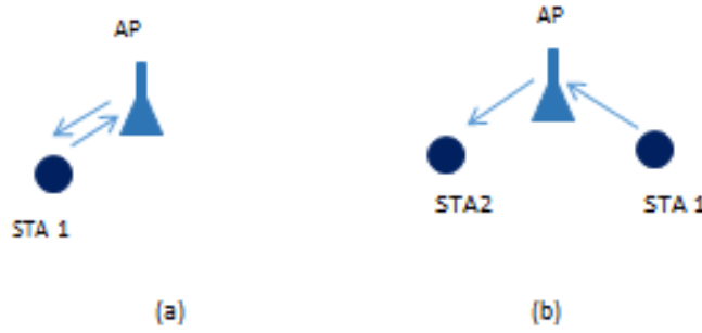
Fig. 1. Full Duplex transmission: (a) Bidirectional, (b) Unidirectional.
