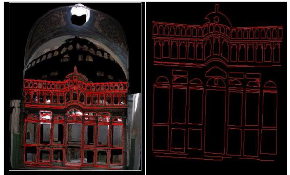
Figure 20. Drawing from point clouds of CC' section
