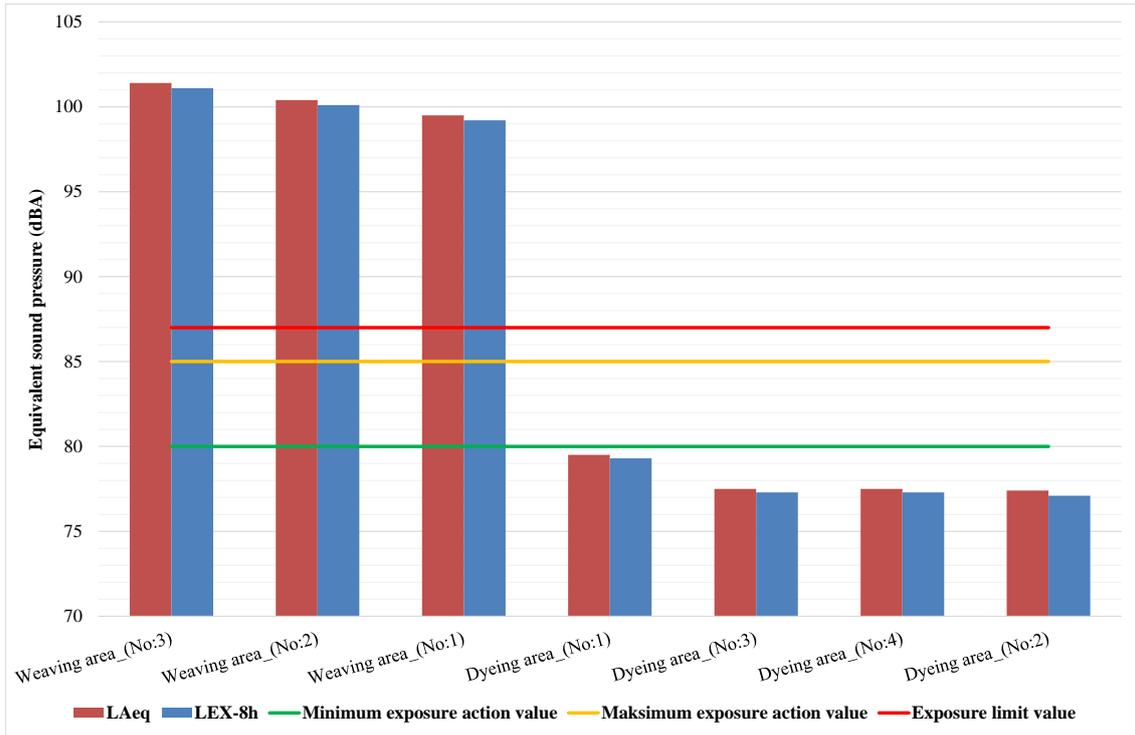
Figure 3. Noise levels during operations in the textile plant.
