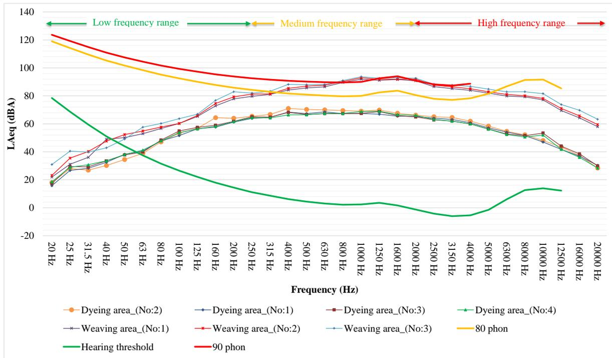
Figure 5. Frequency distribution of noise levels during operations of the textile plant.
