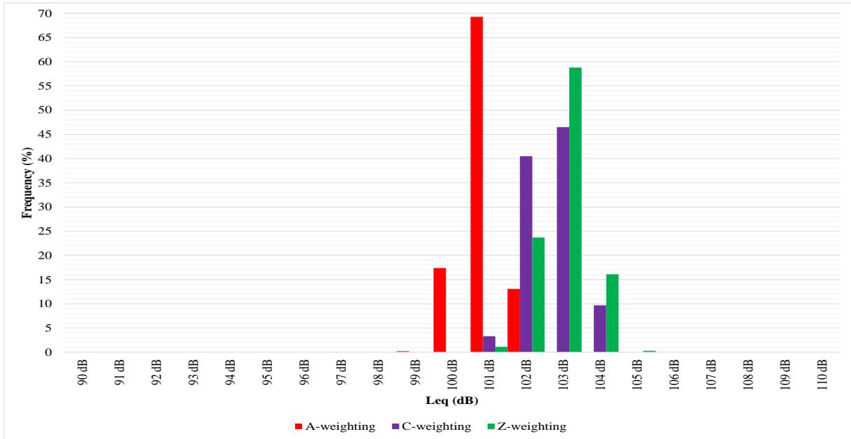
Figure 4b. Dyeing/finishing division noise histogram
