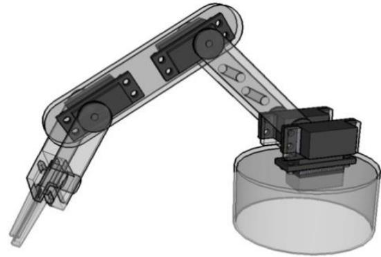
Figure 5. A robotic arm made of servo motors
