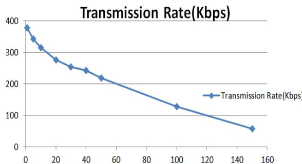
Figure 17. Graph showing transmission rate with respect to Distance
