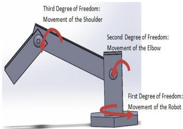
Figure 10. Robot arm degree of freedom
