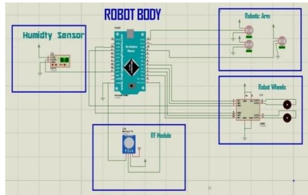
Figure 3. Circuit Diagram of the Robot Body
