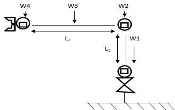
Figure 8. Robotic Arm Free Body Diagram.
