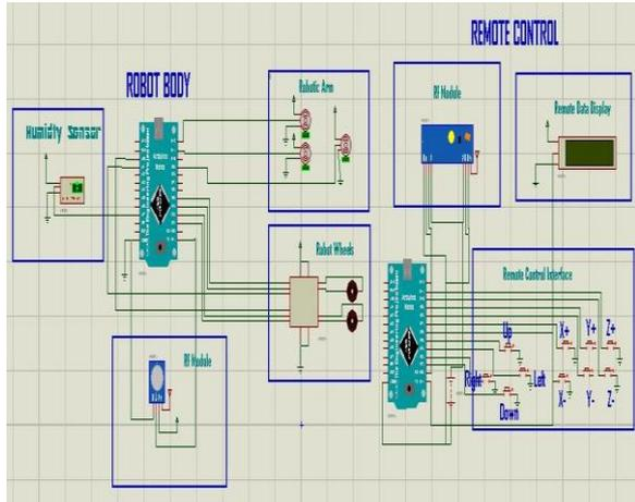
Figure 7. Monitoring Robot Overall System Circuit Diagram
