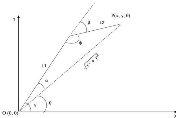
Figure 9. Robotics arm on X Y plane
