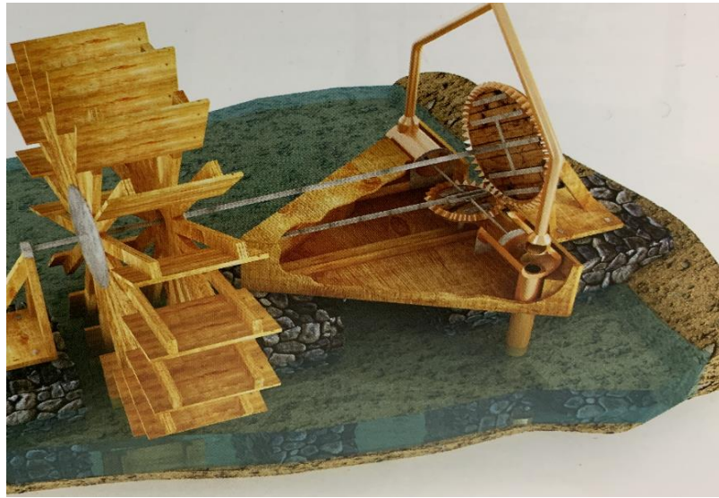
Figure 3. water-raising machine (include Piston, cylinder, valve) ([6])
