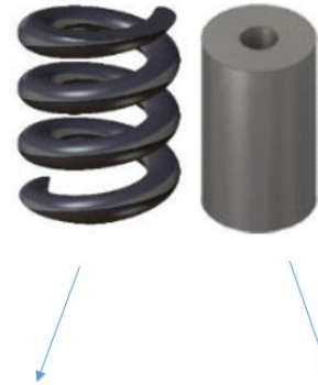
Metallic damper spring b) Rubber damper spring
