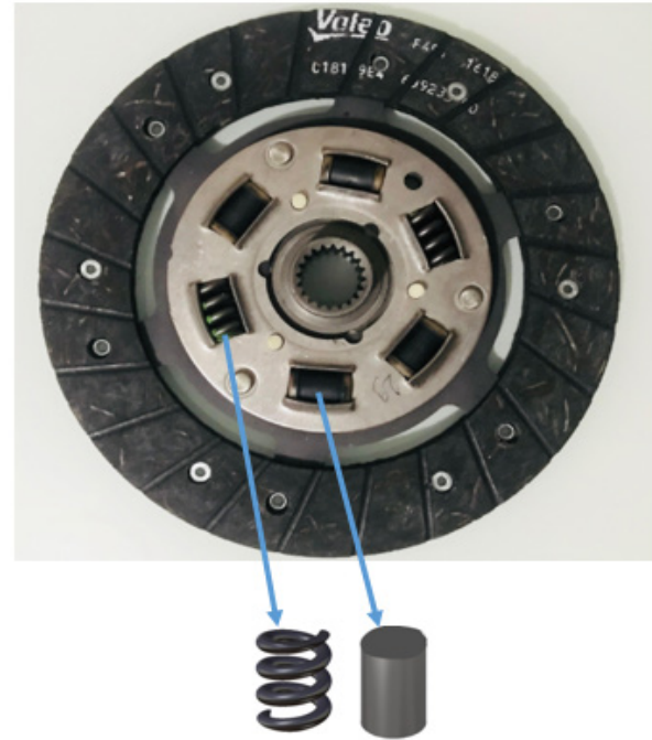
Figure 5. The prototype of hybrid damper clutch disc
