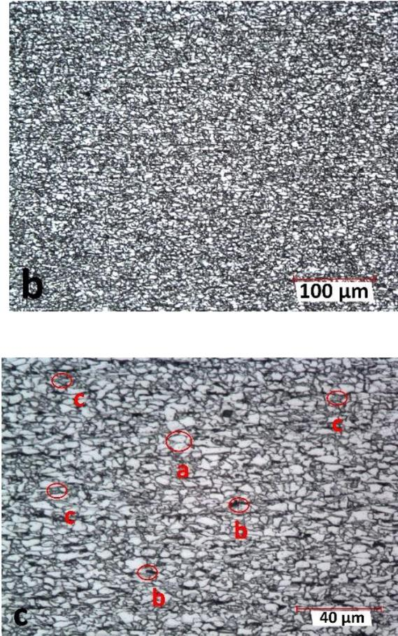
**Figure 2.** Microstructure of Nb-added microalloyed steel (EN 10149-2:2013 S355MC (QStE 380TM)) ( in figure c a : ferrite b : pearite c : NbC )
