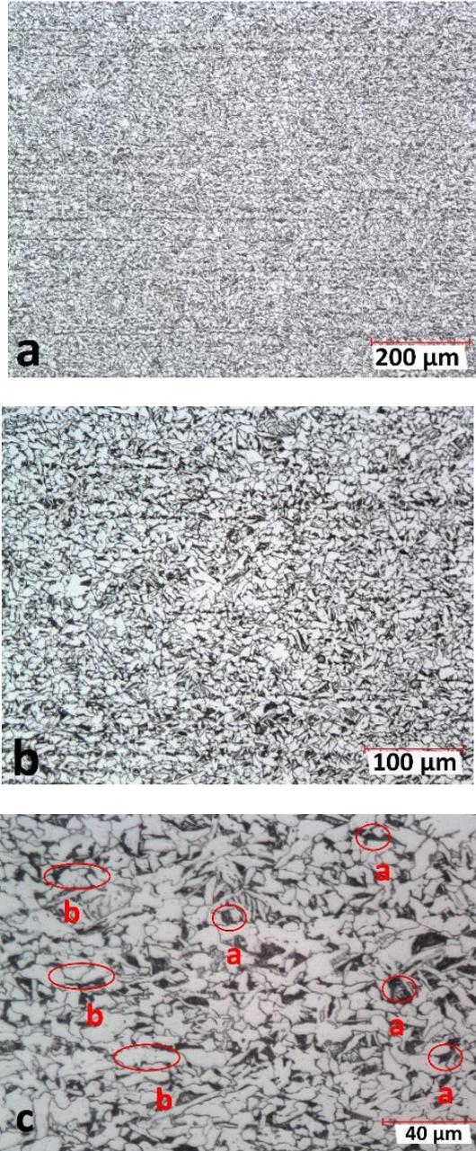
**Figure 1.** Microstructure of non-microalloyed steel (EN 10025-2:2004 S275JRC (RSt37-2)) ( in figure c a : acicular ferrite b : pearite)
