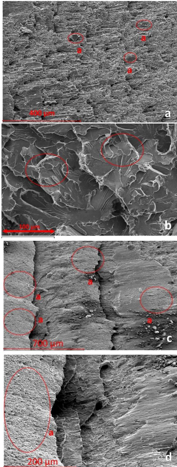
**Figure 4.** Fracture surfaces of samples (a, b Nb-added steel, c and d Nb-Ti added steel)
