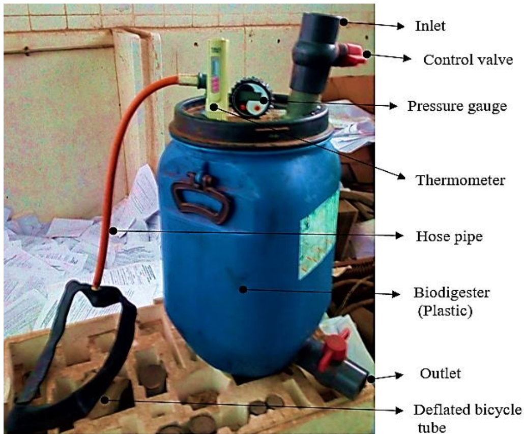
Figure 1. Experimental set-up for anaerobic digestion
