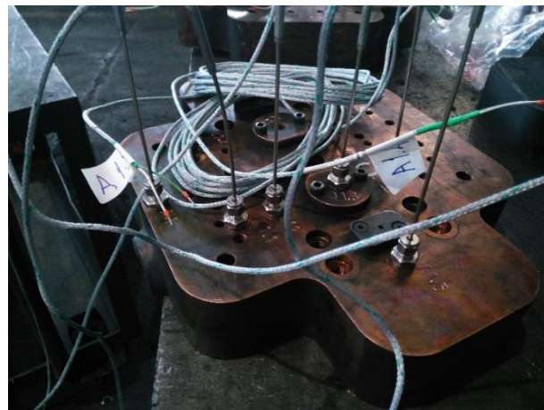
Figure 3. Existing production mold and assembled thermocouples
