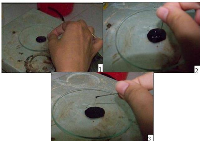
**Figure 5.** Spinnability test for lignin solutions
