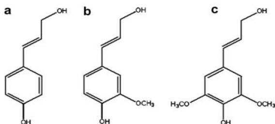
**Figure 1.** (a) p- Kumaryl alcohol, (b) Coniferyl alcohol (c) sinapyl alcohol [12], [14].
