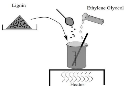
**Figure 4.** Schematic drawing figure of a preparing lignin-ethylene glycol blend.
