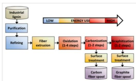
**Figure 3.** Lignin Carbon Fiber Extrusion [26].
