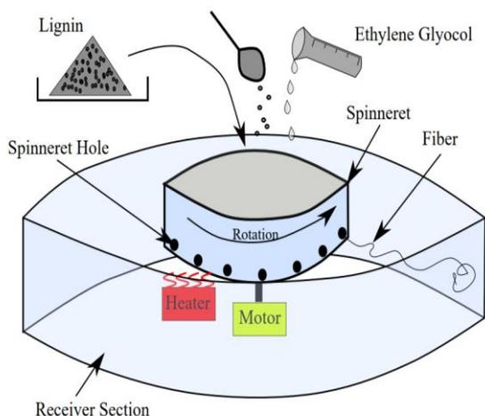
**Figure. 6** Schematic Drawing of Experimental Melt Spinning Method.
