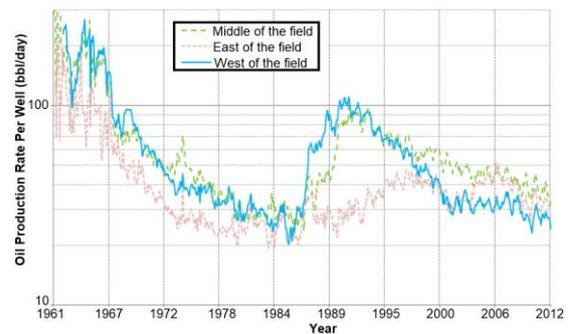
**Figure 4.** Regional average oil production rates per well in Batu Raman Oil Field [9].
