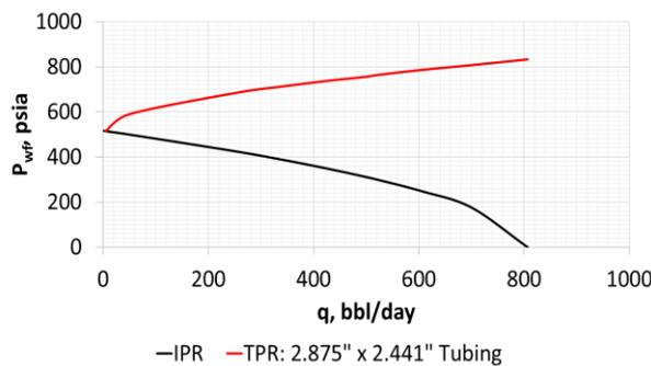
**Figure 6.** IPR-TPR curves constructed for Case 2 in this study.
