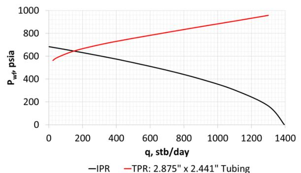
**Figure 7.** IPR-TPR curves constructed for Case 3 in this study.
