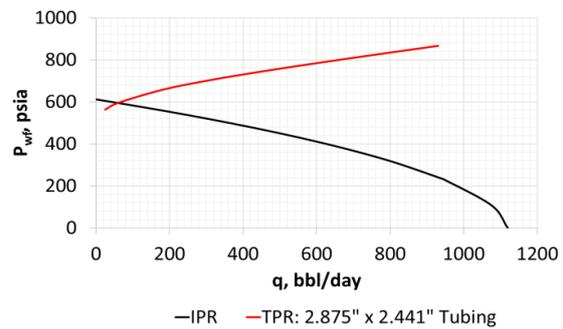
**Figure 5.** IPR-TPR curves constructed for Case 1 in this study.
