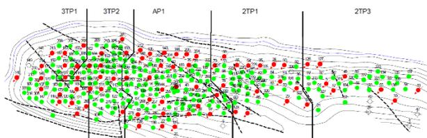
**Figure 2.** Garzan Structure Map of Bati Raman Oil Field (Green circles: production wells; Red circles: injection wells) [7].
