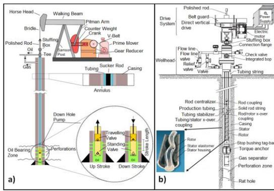
**Figure 3. a.** Sucker Rod Pump (SRP) System (SRP, 2008) **b.** Progressive Cavity Pump (PCP) System [1,25].
