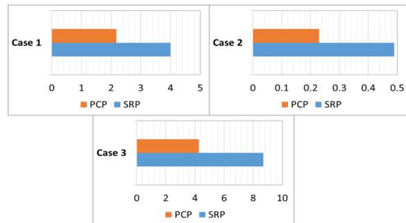
**Figure 8.** Comparison of power requirements in SRP and PCP systems for Case 1 (60 bbl/day), Case 2 (5 bbl/day) and Case 3 (150 bbl/day).
