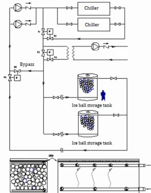
**Figure 5.** Spherical encapsulated thermal energy storage system (Iceball, [15])
