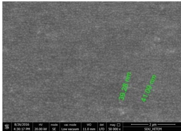
**Figure 2.** The crystallite size obtained in SEM images
