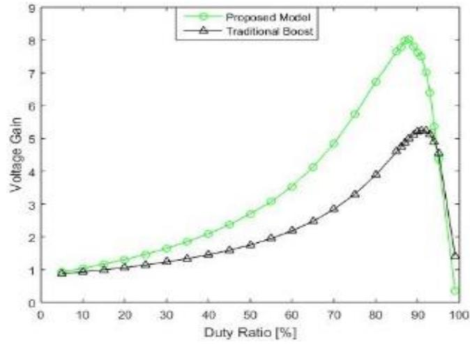
FIGURE 5. Voltage gain comparison for  $V_i = 5$  V,  $R/R_L = 125$
