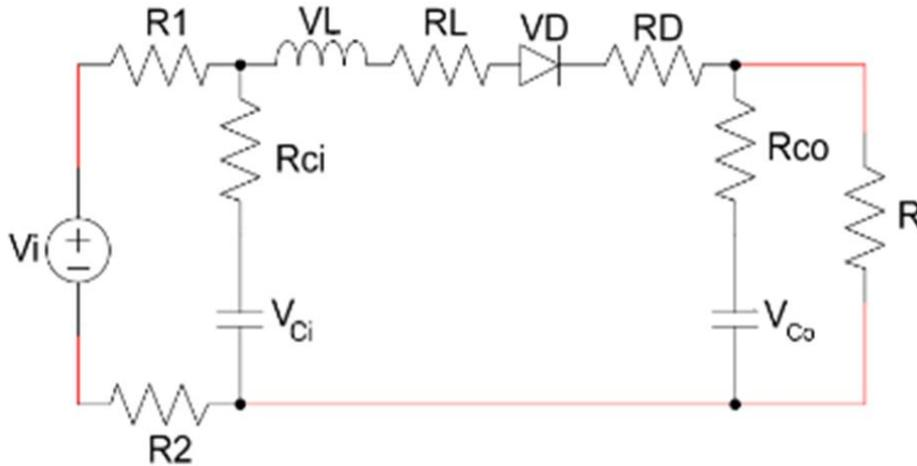
FIGURE 2.  $T_1$  &  $T_2$  on,  $T_3$  &  $T_4$  off,  $C_i$  is being charged from the voltage source
