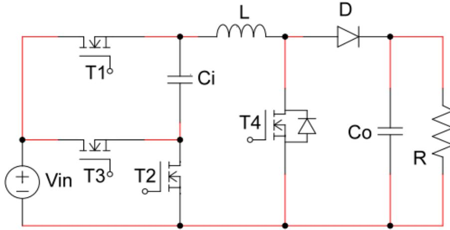
FIGURE 1. The modified Boost converter circuit
