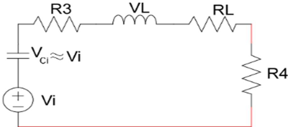
FIGURE 3.  $T_3$  &  $T_4$  on,  $T_1$  &  $T_2$  off,  $C_i$  is acting as a secondary voltage source
