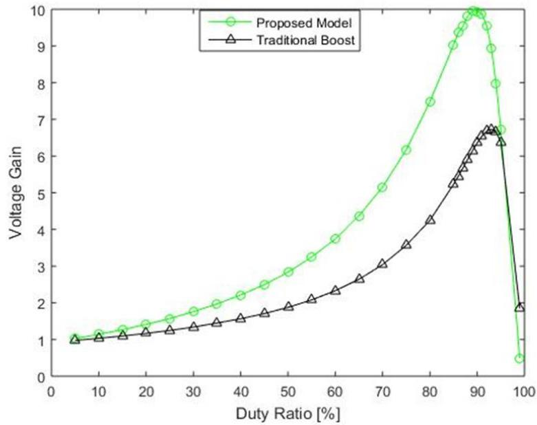
FIGURE 4. Voltage gain comparison for  $V_i = 12$  V,  $R/R_L = 200$
