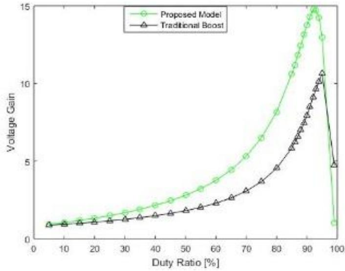
FIGURE 6. Voltage gain comparison for  $V_i = 5$  V,  $R/R_L = 500$
