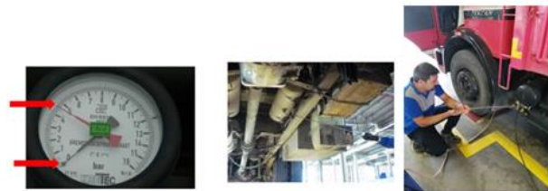
Fig. 4. Emptying of air tanks and pressure control
