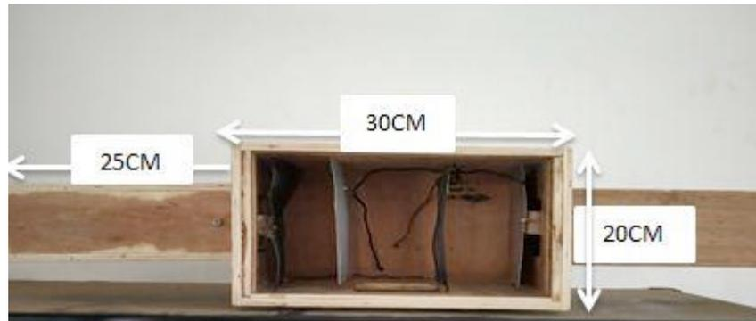
**Figure 1.** Experimental model of ESP
