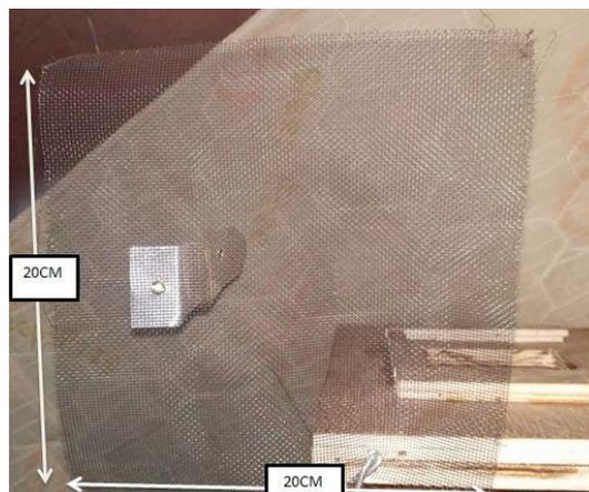
**Figure 2.** Discharge electrodes
