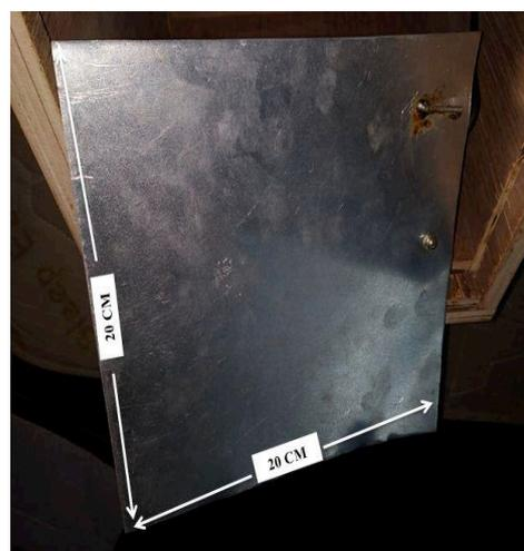
**Figure 3.** Collection electrodes
