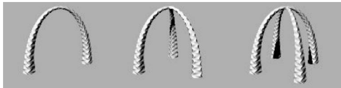
Fig.16. Pottery material wire print can make one-curve path to print, continuously extruding not only enhance the stable of structure, but
