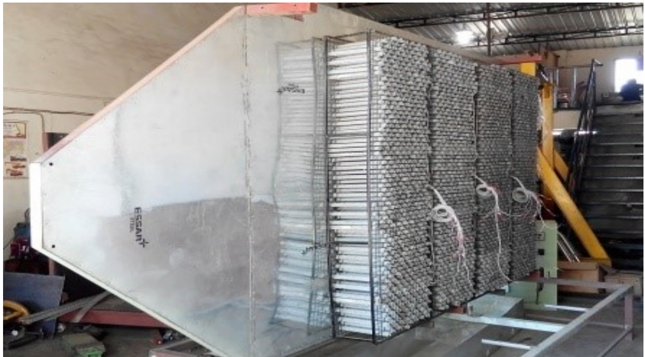
Figure 2. Internal view of cooling tower
