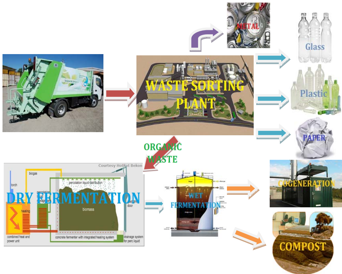
Figure 1: The flow scheme of a solid waste recycling, disposal and energy production facility.
