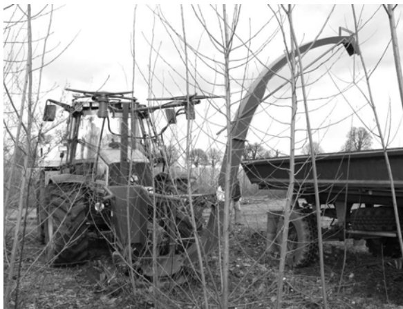
Figure 5. A new development of a 1 row-tractor-mounted cutter chipper (ATB)
