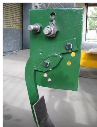
Figure 2. Blade rotation mechanism to achieve desired rake angle
