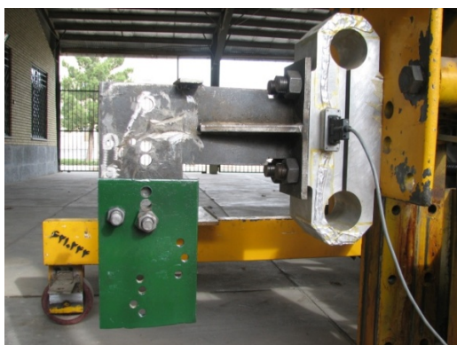
Figure 3. the octagonal ring transducer connected to the tool carriage
