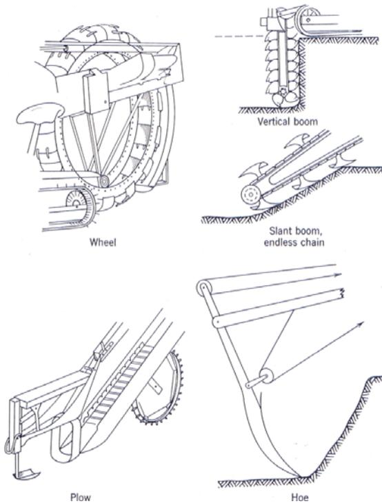
**Figure 2. General classes of trenching machines (Frevert et al, 1955)**
