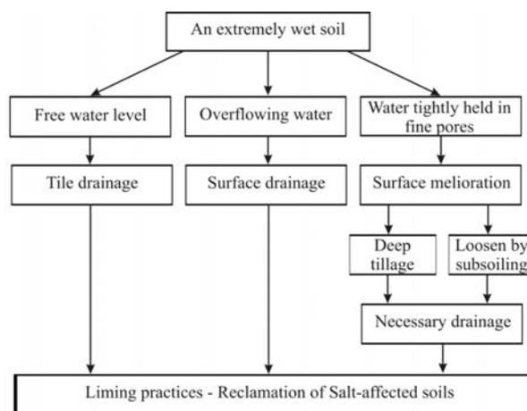
Figure 1. The use of modern drainage methods depending on soil moisture (Wolff, 1987)
