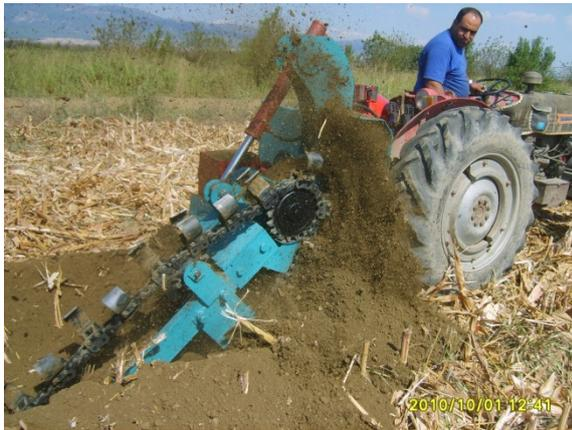
**Figure 3 a. Engagement of the trencher in field (without security frame attached)**
