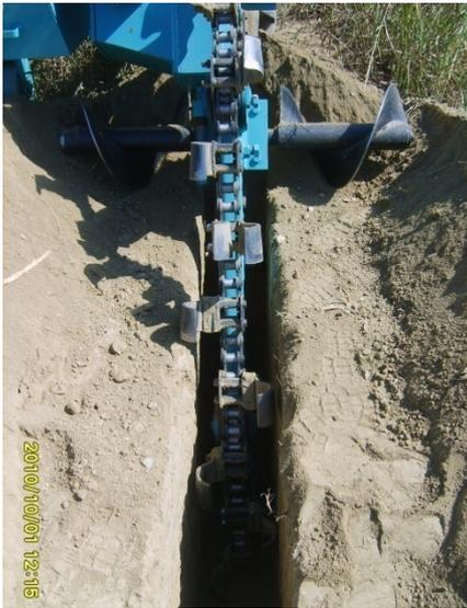
**Figure 6. Spiral conveyors**
