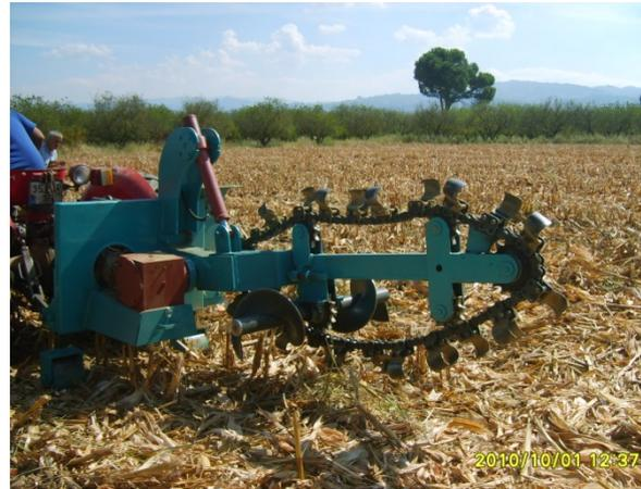
**Figure 4. Linking Slant-boom type endless-chain to main frame**
