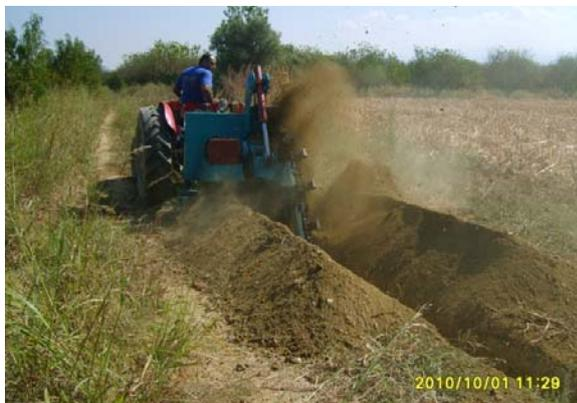
**Figure 7. Trencher, spreading stones and soil without safety frame**
