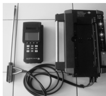
Figure 2. Flue gas analyzer
