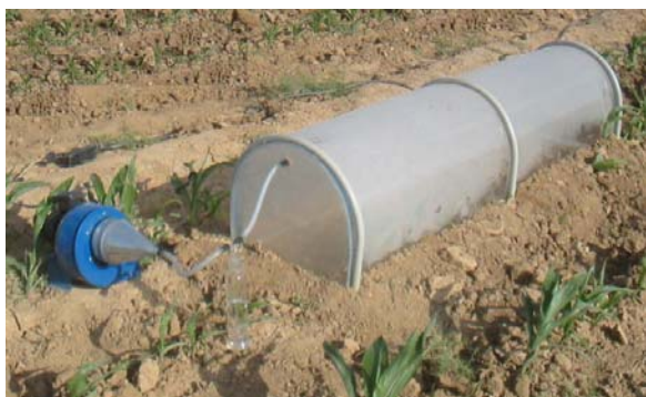
Figure 3. The system for measuring nitrogen loss
