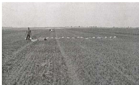
Figure 8. Determination of the transverse straw/chaff distribution after combine harvesting using the collection containers (60 cm Ø round or 50 * 50 cm square grids)
