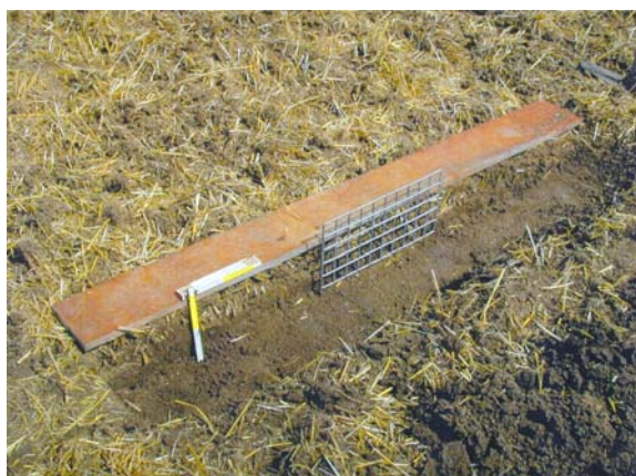
Figure 10. Determination of straw distribution on the surface or in the soil profile by using the 4.5 * 4.5 cm gridiron system.
