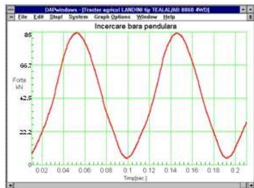
Figure 7. The force-time diagram for the traction bar fig. 6 - at 250.000 cycles fig. 7 - at 427.000 cycles
