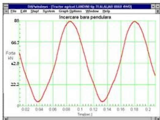
Figure 5. The force-time diagram for the traction bar fig. 4 - at 10.000 cycles; fig. 5 - at 100.000 cycles
