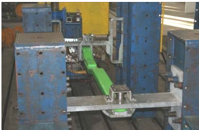
Figure 3. The fitting realized on the hydropulse installation for the mechanical test of the tractor's traction bar
