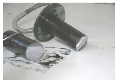
Figure 10. Breakage of the connection bolt for the mechanical test of the traction bar from the ZIMBRU 2200 tractor (after 427.000 cycles)
