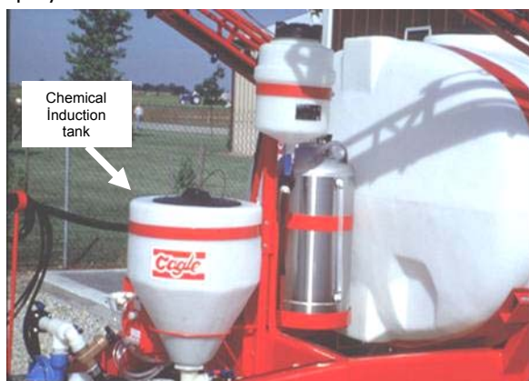
Figure 1. Modern sprayers are equipped with a chemical induction tank and several other smaller tanks
