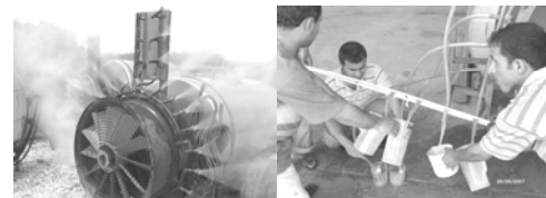
Fig. 5. Inspection and function tests of orchard sprayers
