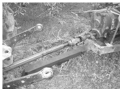
Fig. 6. Inspection the PTO shaft guard
