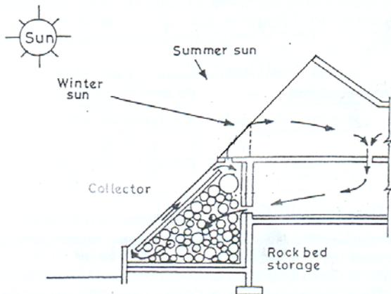
Fig. 2. The rock bed-passive solar system
