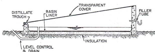
**Fig. 6. The continuous passive solar water still**
