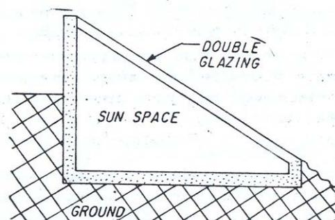
**Fig. 1. The pit type structural design**
