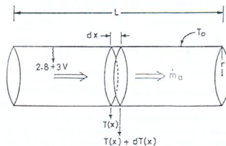
Fig. 4. Flow direction through an earth-air tunnel
