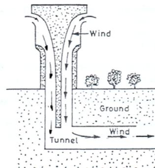
Fig. 3. The cross sectional view of an earth tunnel and wind tower
