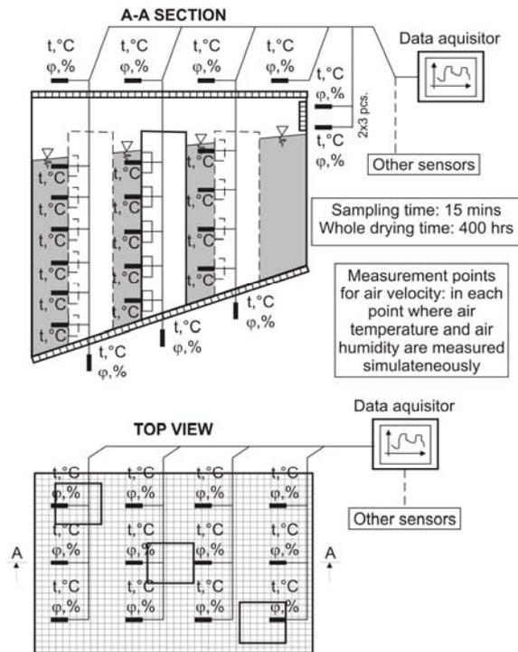
**Figure 2. Assembly of the main data acquisition system for measuring the temperature and humidity of drying air and the temperature of drying material**
