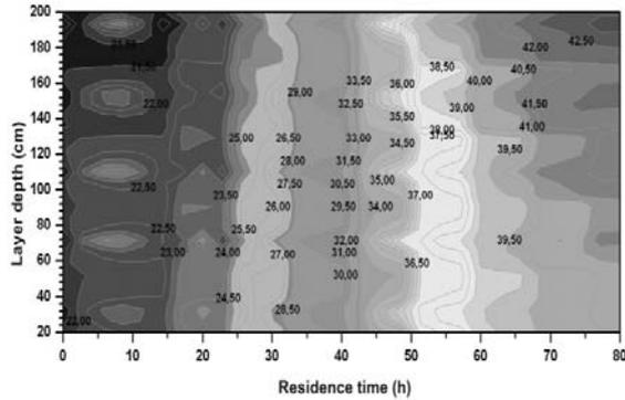
Figure 5. Characteristic temperature map of the corn-cob as functions of the layer depth and the drying time
