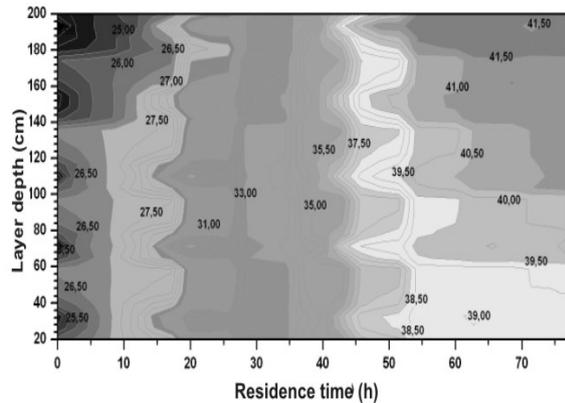
Figure 6. Temperature of the bulk as functions of the layer depth and the drying time
