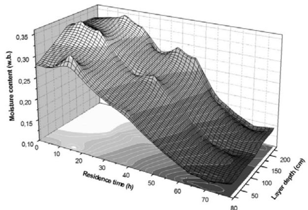
**Figure 4. Typical integrated moisture content of corn-kernels as functions of the drying time and the layer depth**
