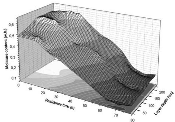
**Figure 3. Typical integrated moisture content of the corn-cob as functions of the drying time and layer depth**
