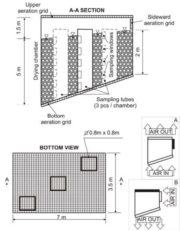
**Figure 1. Structure of the drying chamber (A: 1<sup>st</sup> setup of aeration; B: 2<sup>nd</sup> setup of aeration)**
