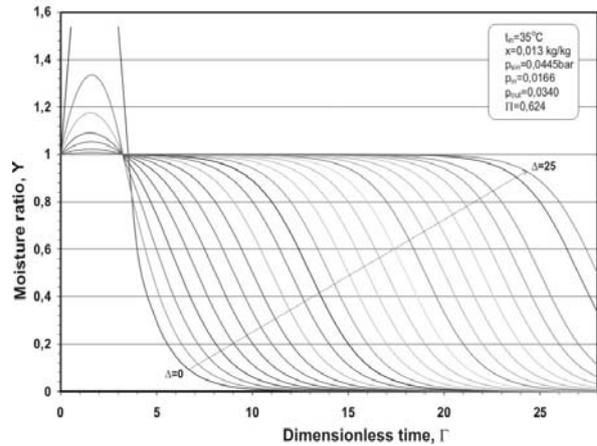
Figure 7. Modified Hukill-curves based on the seed-corn-cob drying conditions without changing the drying air direction
