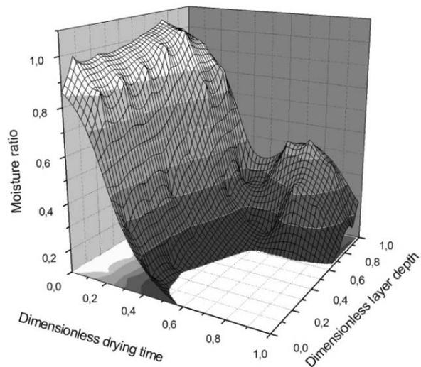
Figure 8. The local overdrying as the influence of the delayed change of drying air direction
