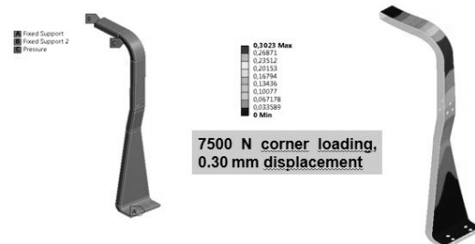
Figure 5. Analysis of alternative design 2 (Filled structure)
