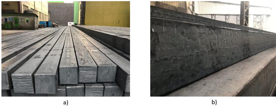
Figure 5. Pictures of some billets cast with the new mold and secondary cooling scenario a) general and b) longitudinal
