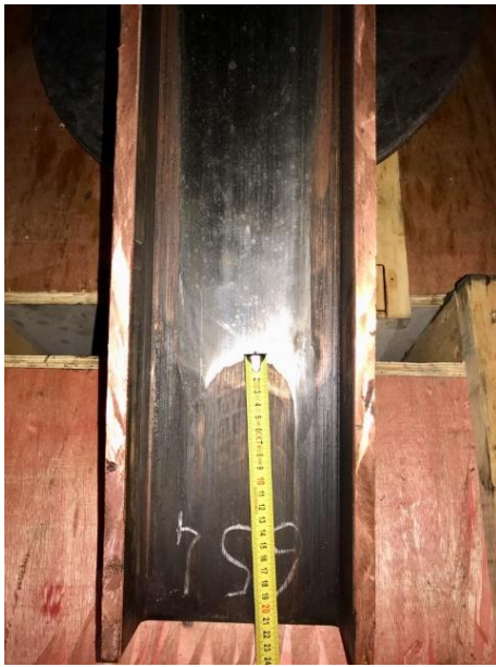
Figure 12. The view of inner wall of the mold after an operation of casting 654 heats
