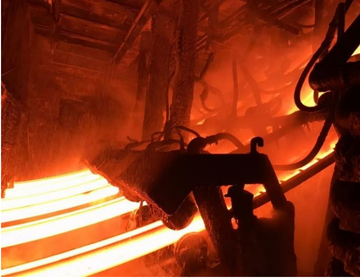
Figure 3. A picture from the secondary cooling zone during the continuous casting
