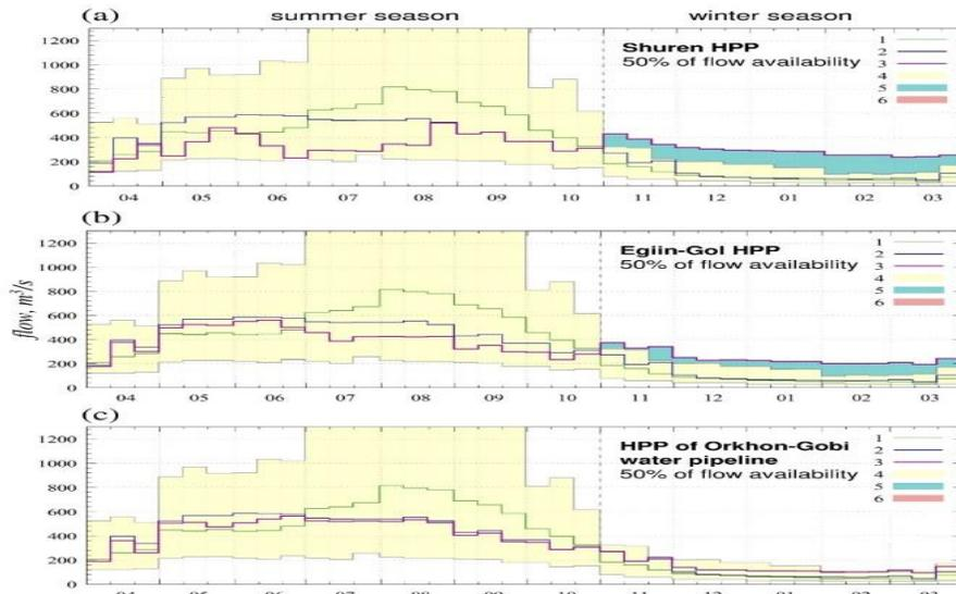
**Figure 4.** Change in the Selenga river flow under regulation of Shuren HPP (a) Egiin-Gol HPP (b) HPP of Orkhon-Gobi water diversion system (c) at Naushki station for 50% of flow availability (1 – norm; 2 – environmental flow; 3 – regulated flow; 4 – range of natural flow changes; 5 – upper level overrange of environmental flow; 6 – lower level overrange of environmental flow).
