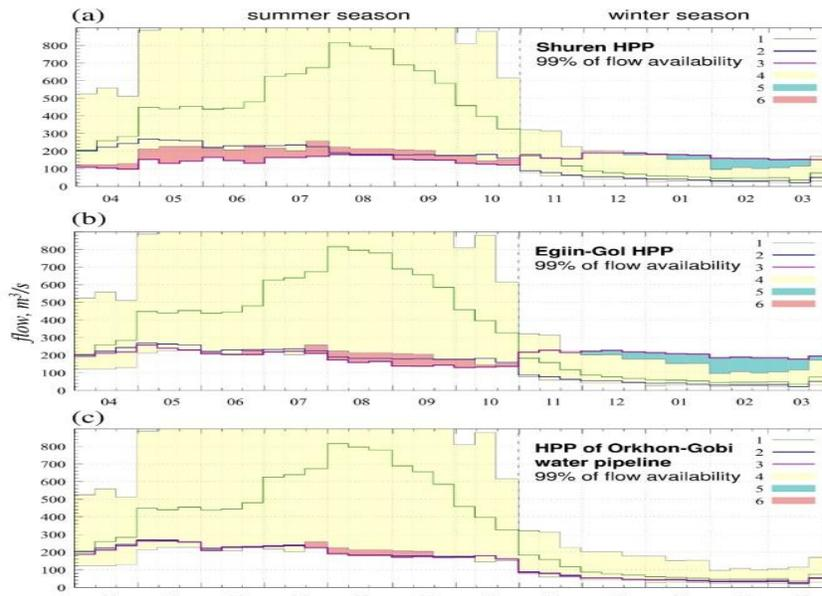
**Figure 5.** Change in the Selenga river flow under regulation of Shuren HPP (a) Egiin-Gol HPP (b) HPP of Orkhon-Gobi water diversion system (c) at Naushki station for 99% of flow availability (1 – norm; 2 – environmental flow; 3 – regulated flow; 4 – range of natural flow changes; 5 – upper level overrange of environmental flow; 6 – lower level overrange of environmental flow).
