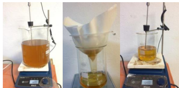
Fig. 2. Heating and filtration of waste sunflower oil and removal of water particles
