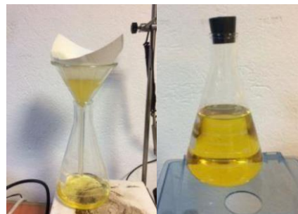
Fig.5. Filtering and storage of biodiesel
