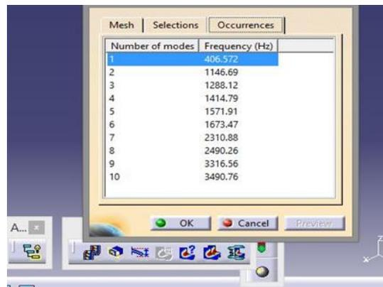
Figure 16. Frequency at different modes
