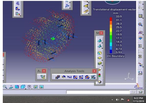
Figure 14. Translational displacement (Titanium)
