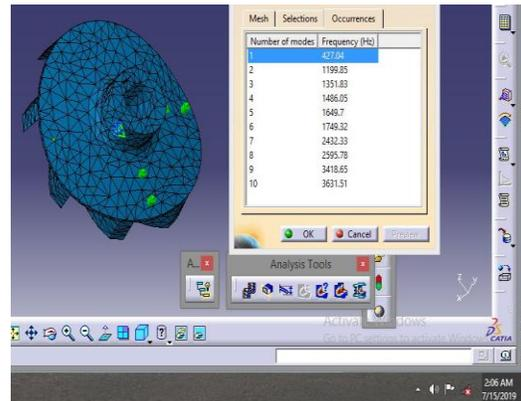
**Figure 12.** Freq of the impeller at different modes
