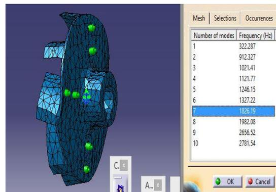
Figure 8. Shape of the 7<sup>th</sup> mode
