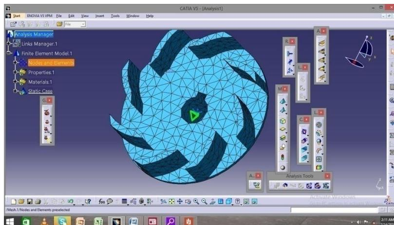
Figure 2. Meshed model of the impeller using CATIA V5 R20
