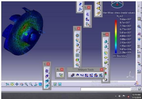
**Figure 9.** Von-Mises stress of water pump impeller
