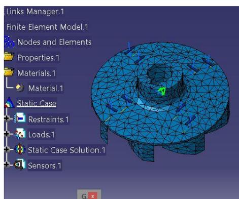
Figure 19. Deformation of the impeller
