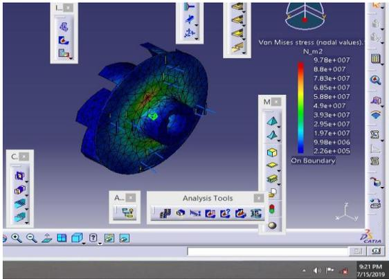
Figure 13. Von-mises stress of the impeller
