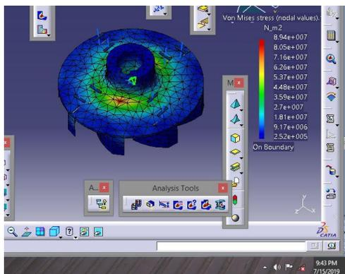
Figure 17. Von-Mises stress of the impeller (bright plastic)
