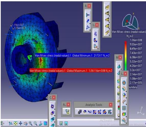
Figure 3. Von-mises stress of water pump impeller
