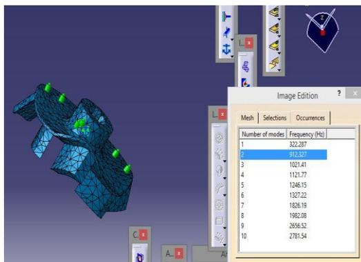
Figure 7. Shape of the 2<sup>nd</sup> mode
