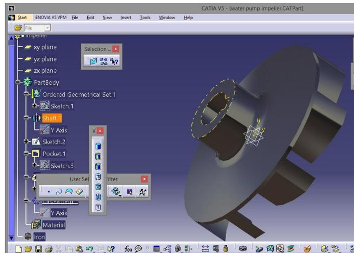
Figure 1. Solid model of the water pump impeller
