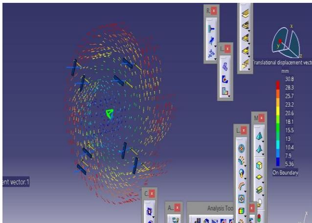
Figure 5. Translational displacement vector of the impeller (aluminium)
