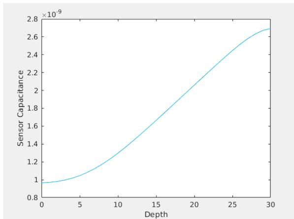
**Figure 8.** Sensor Capacitance versus Submerged Depth.
