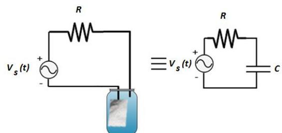
**Figure 2.** The sensor feeding circuit and its equivalent circuit.
