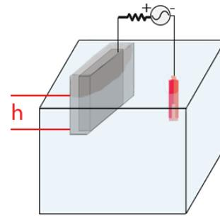
Figure 5. System topology when its electrode is at the submerged height  $h$ .
