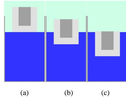
Figure 6. System topology drawn in Matlab at three different submerged heights: a)  $h = \Delta y$ , b)  $h = 15\Delta y$ , and c)  $h = 30\Delta y$ .
