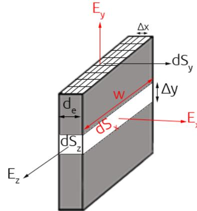
**Figure 4.** The differential areas used to calculate the electrode charge.
