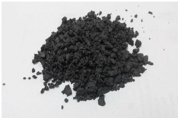
Fig. 1. View of ferro-chromium slag aggregate
