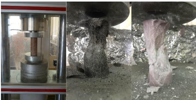
Figure 7 The pressure test of the filled composites
