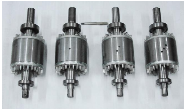
Figure 4. Healthy rotor and rotors with one, two and three broken bars (Pezzani et al., 2014)
