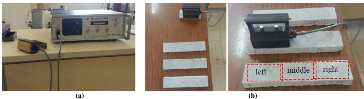
Figure 2. a) Thermal conductivity test setup, b) Measurement method.
