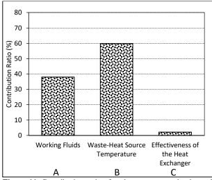
**Figure 11.** Contribution ratio of each parameter to the thermal efficiency
