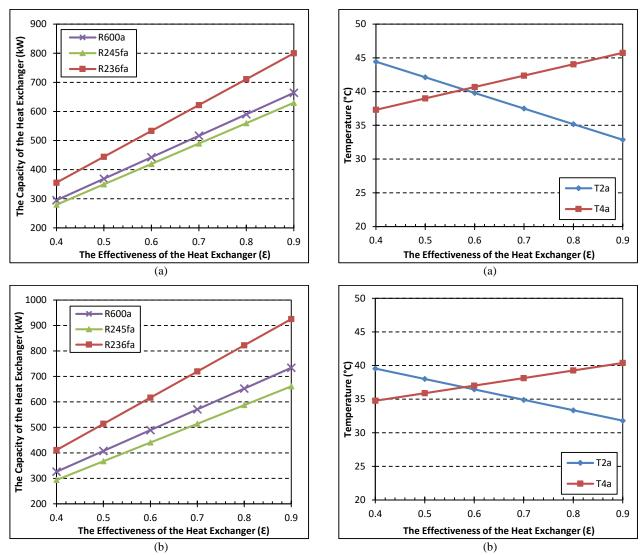
**Figure 8.** The change of heat exchanger capacity according to the effectiveness of the heat exchanger for different waste-heat source temperatures (a)  $T_s$ =100°C (b)  $T_s$ =80°C
