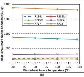
**Figure 5.** The change in the amount of heat exhausted from condenser in order to obtain 1MW turbine work, depending on the waste-heat source temperature
