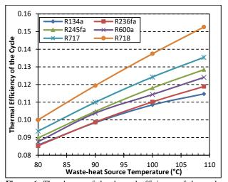
**Figure 6.** The change of the thermal efficiency of the cycle depending on waste-heat source temperature
