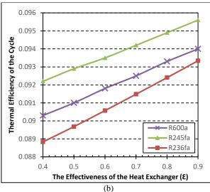
**Figure 10.** The variation of cycle thermal efficiency according to the effectiveness of the heat exchanger at different waste-heat source temperatures. (a)  $T_s=100$ °C (b)  $T_s=80$ °C
