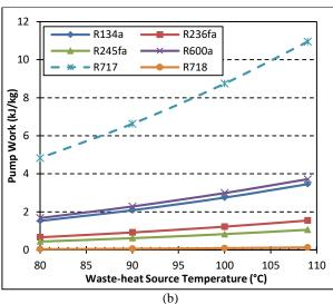
**Figure 4.** The change of necessary pump work required to obtain 1MW turbine work, depending on the waste-heat source temperature
