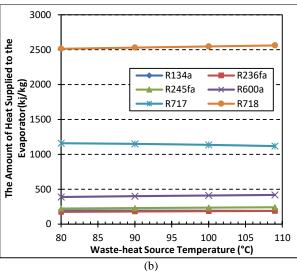
**Figure 3.** The change in the amount of heat that is transferred to evaporator in order to obtain 1MW turbine power, depending on the waste-heat source temperature
