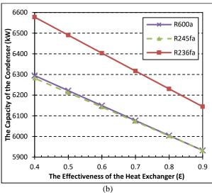
**Figure 7.** For 100°C of waste-heat source temperature, the change in evaporator and condenser capacities depending on the effectiveness of the heat exchanger (a) the capacity of the evaporator (b) the capacity of the condenser.
