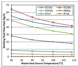
**Figure 2.** The change of the working fluid flow rates, necessary to produce 1MW turbine work, depending on the waste-heat source temperature
