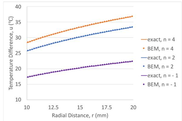
**Figure 3.** Comparison of exact and BEM results for  $n = -1$ ,  $n = 2$  and  $n = 4$ .
