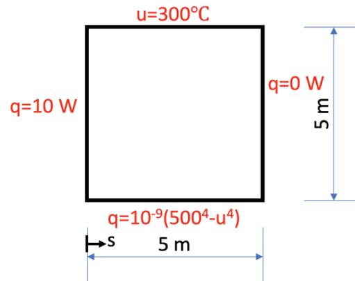
**Figure 7.** The square plate domain with dimensions and boundary conditions
