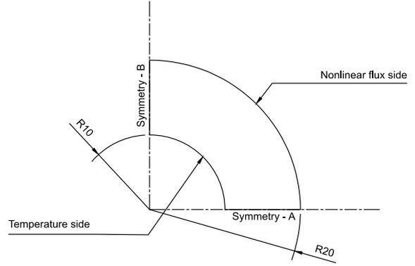
**Figure 2.** The quarter model for solution of the problem. The numerical results will be presented in three cases, with  $n = 2$ ,  $n = -1$  and  $n = 4$ .
