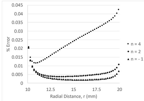
**Figure 4.** Comparison of exact and BEM results for  $n = -1$ ,  $n = 2$  and  $n = 4$
