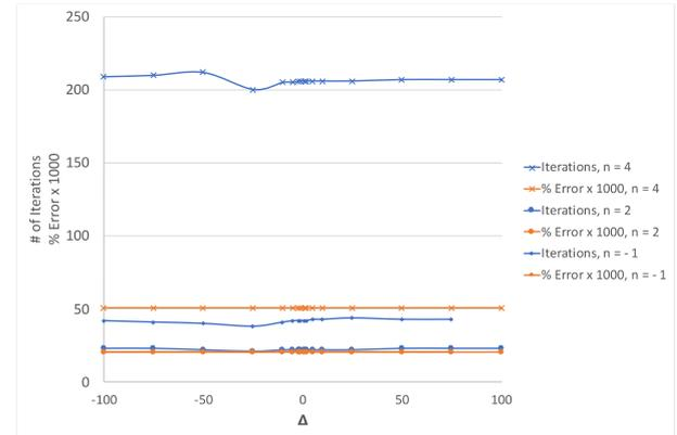
**Figure 6.** Sensitivity of the solution accuracy (% Error x 1000) and the number of iterations to obtain the solution with respect to  $\Delta$
