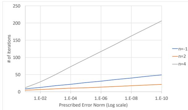
**Figure 5.** Number of iterations to obtain solution for  $n = -1$ ,  $n = 2$  and  $n = 4$
