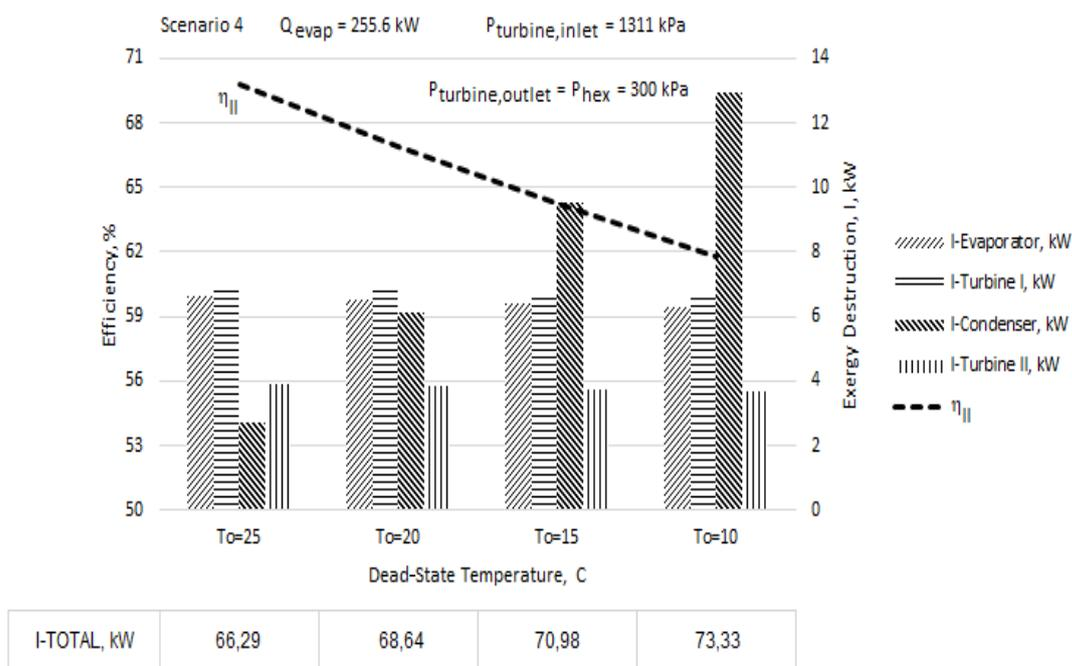
**Figure 9.** Evaluation of the effect of dead-state temperature for Scenario-4.
