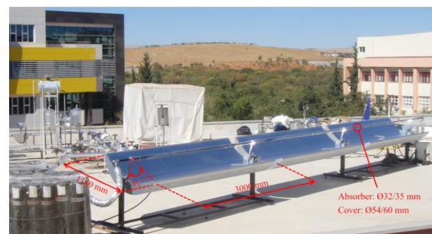
Figure 1. Testing setup and collector geometry.
